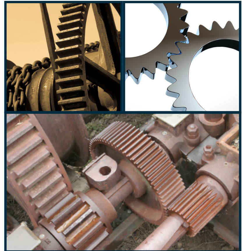
In-Running Nip Points (the point where two gears mesh or where conveyor belts and rollers meet) are frequent areas for injuries and must be guarded for safety.
